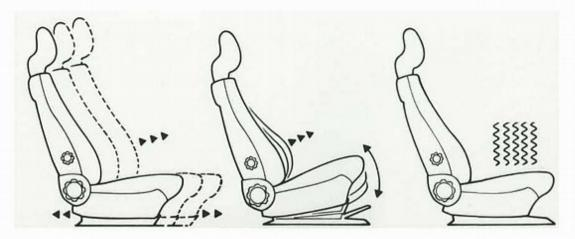
Seat adjustment for proper driving position is extremely important both for comfort and safety. Front seats can be adjusted through an extraordinary range of positions to help ensure that the driver and passenger stays comfortable, alert and refreshed - even after many hours on the road.
