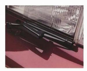
Headlight wiper/washers help maintain headlamp efficiency by removing road dirt. They operate automatically with activation of the windshield washer feature.
